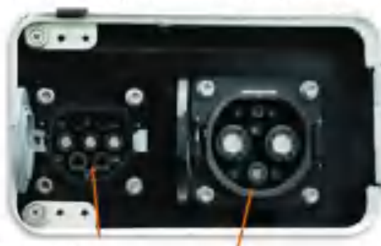
National standard external discharge and slow charging port
